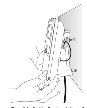
Figure 2-3: attaching the phone to the wall
